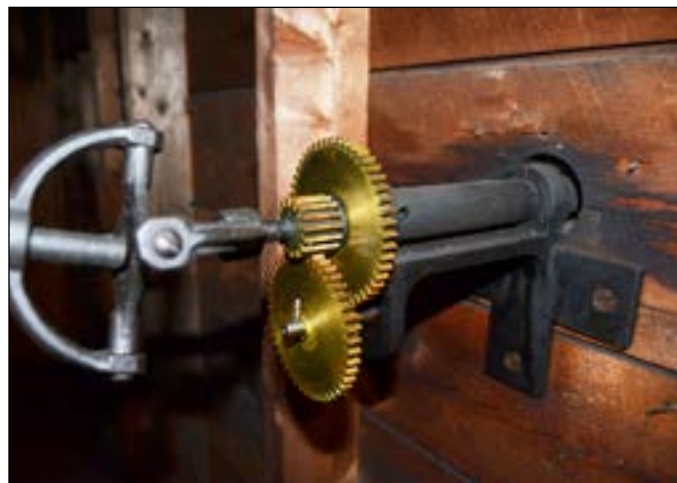
Gearage inside the Belmont Town Clock.
